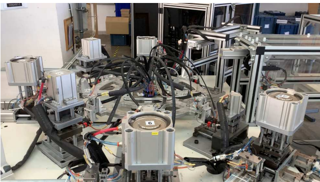
Fig. 2. Control stations on an automatic production line
