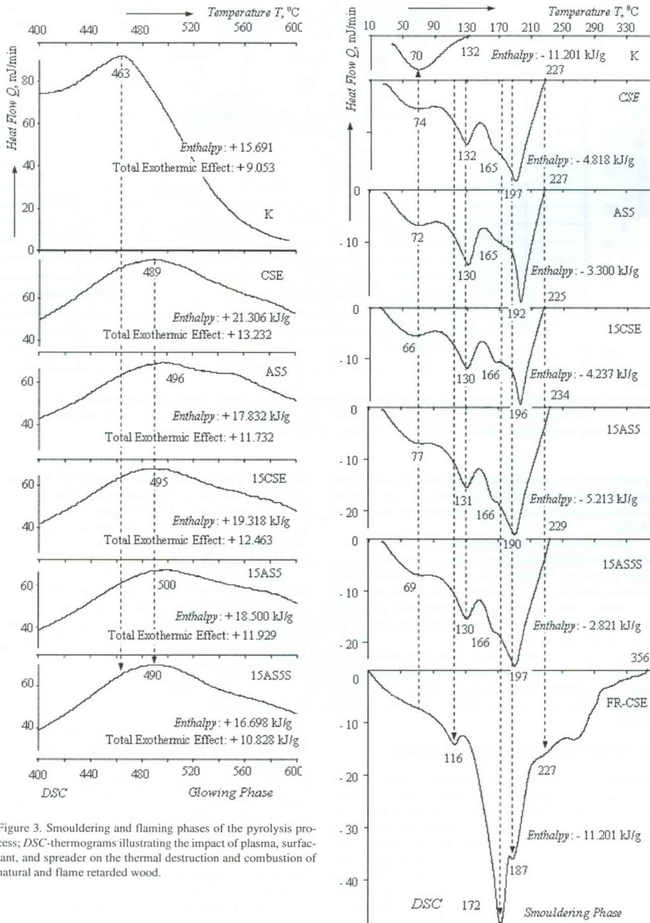
Figure 3. Smouldering and flaming phases of the pyrolysis process; DSC-thermograms illustrating the impact of plasma, surfactant, and spreader on the thermal destruction and combustion of natural and flame retarded wood.
