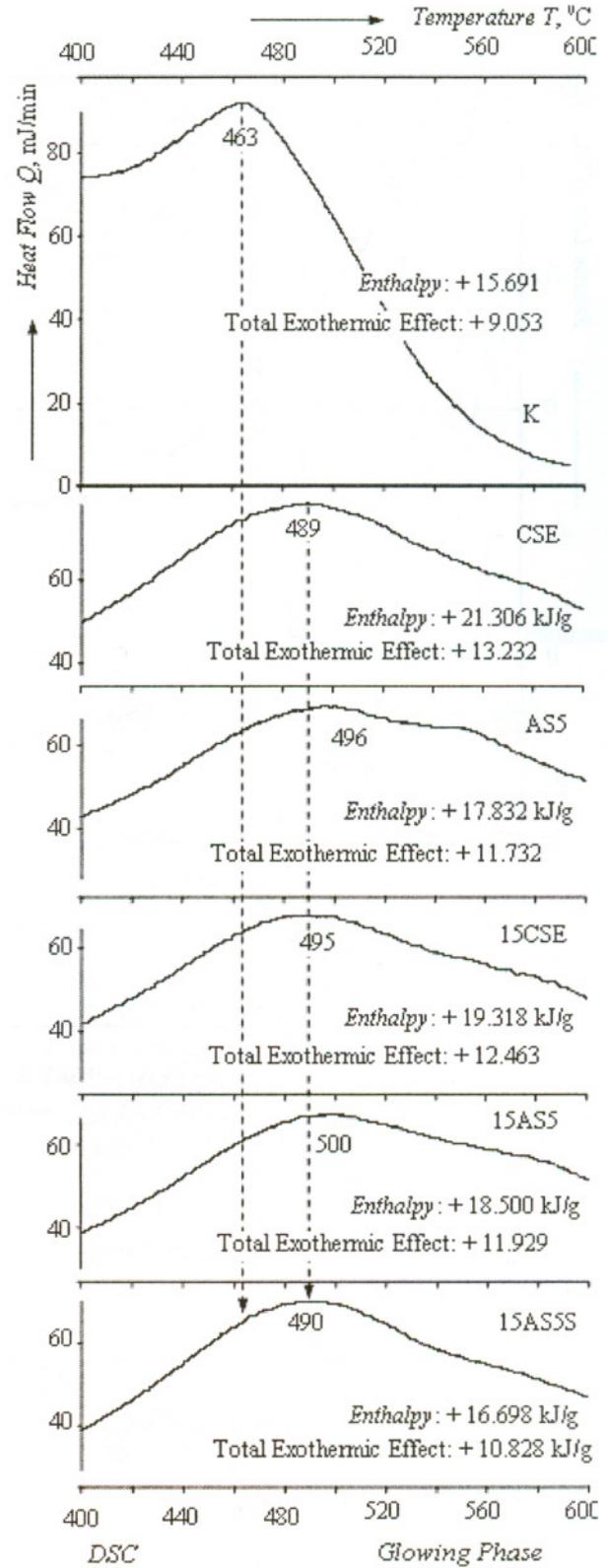
Figure 4. Glowing phase of pyrolysis process - DSC-thermograms; and TG-thermograms of all pyrolysis processes of natural pine wood - K, and different flame retarded woods - CSE, AS5, 15CSE, 15AS5, and 15ASSS.
