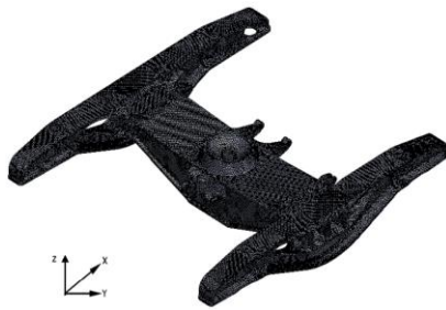
Fig.3. Finite elements mesh of calculation model
