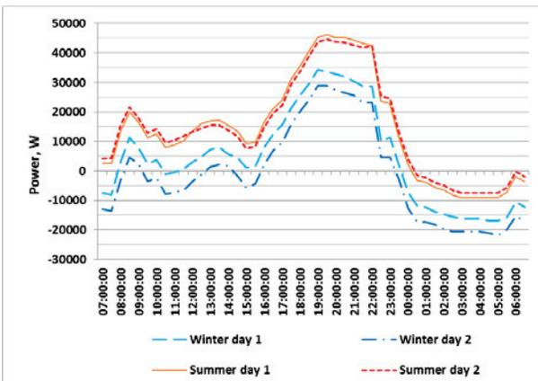
**FIGURE 6.** Resulting load curve of the studied building from the grid point of view
