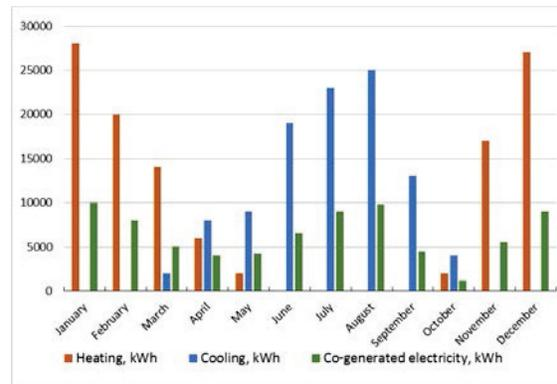
**FIGURE 7.** Monthly estimated heating and cooling energy consumption and the available electrical energy, generated from a CHP system
