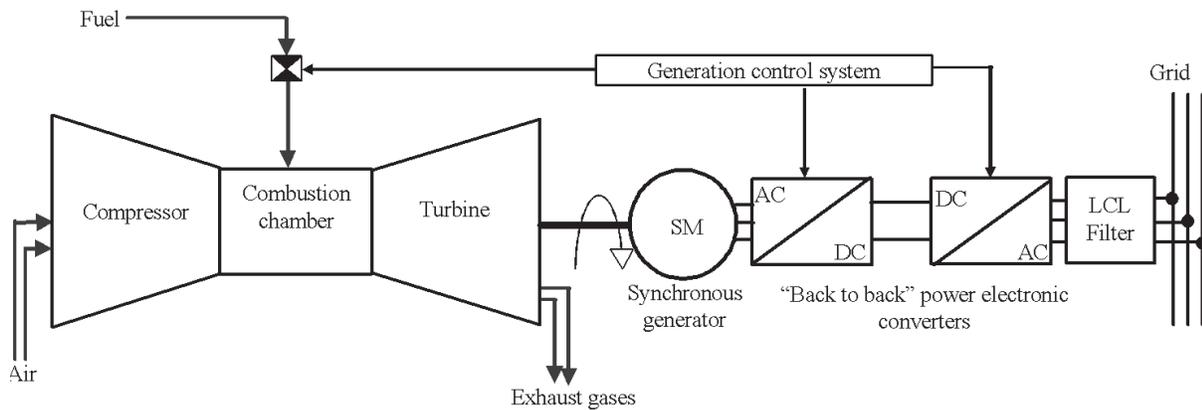
**FIGURE 2.** Schematic representation microturbine CHP
