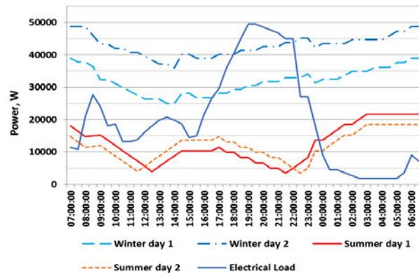
FIGURE 5. Available power from CHP generation and a common daily electrical load curve of the studied building
