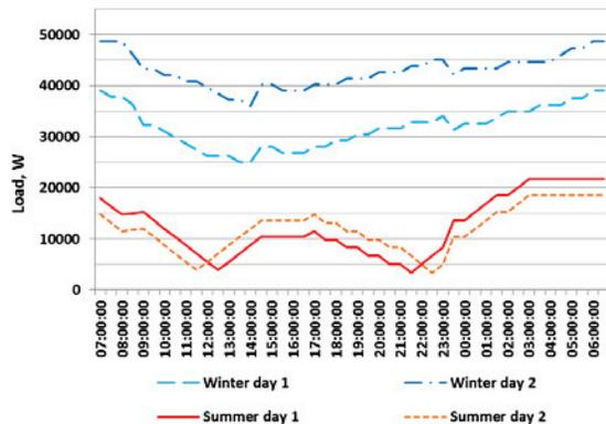
FIGURE 4. Estimated daily thermal load curves (heating or air conditioning) of the building
