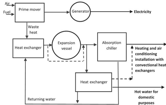
**FIGURE 1.** Bloc diagram of a trigeneration system
