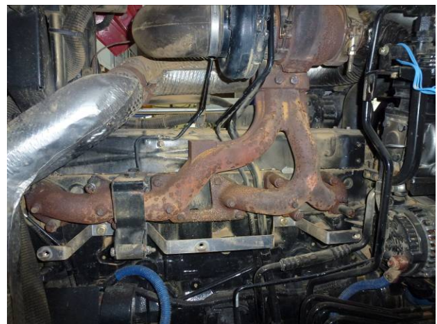
Fig.7 Exhaust manifold and its connection with the turbine housing
