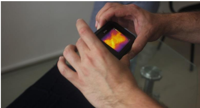
Fig. 5. Temperature measurement and general view of the FLIR C3 thermal camera
