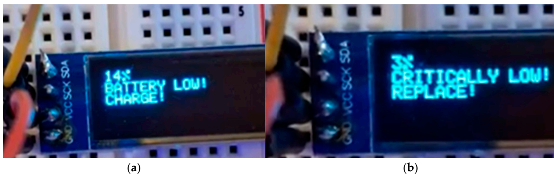
Figure 6. Warnings, displayed on the OLED: (a) Low Voltage event; (b) Critically Low Voltage.
