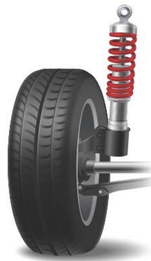
Figure 16. Illustrative example of a car suspension, including the wheel, the spring-damper set and part of the axel. We can imagine the mass of the car attached on top of it.
