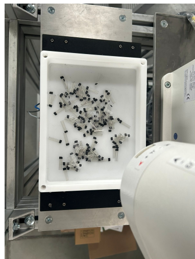
Figure 5. The vibrating platform of the flexible feeder with sample parts in the container.
