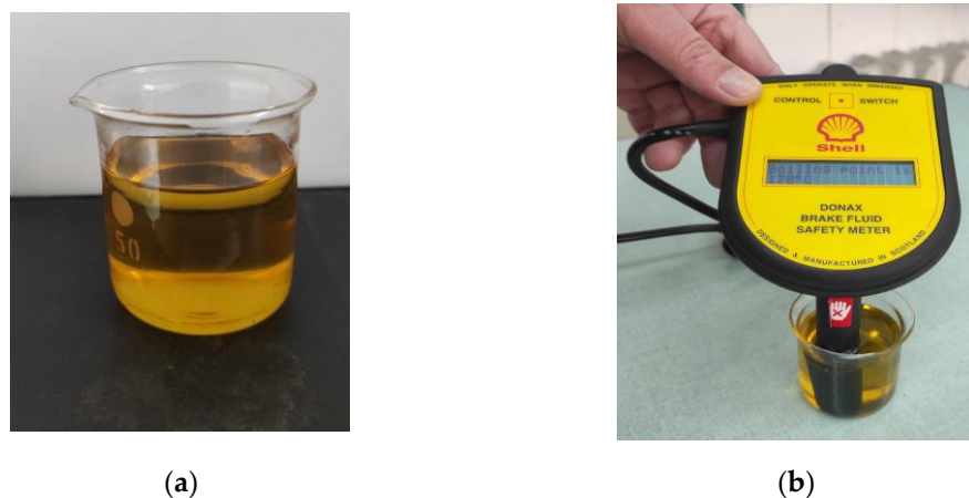
Figure 5. Wet and Dry Boiling point measuring: (a) Glass transparent flask with brake fluid sample; (b) Measuring the boiling point of the sample with Alba Diagnostics brake fluid meter.
