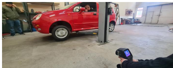
Figure 1. Lifting the vehicle and increasing the temperature of the vehicle's brake discs
