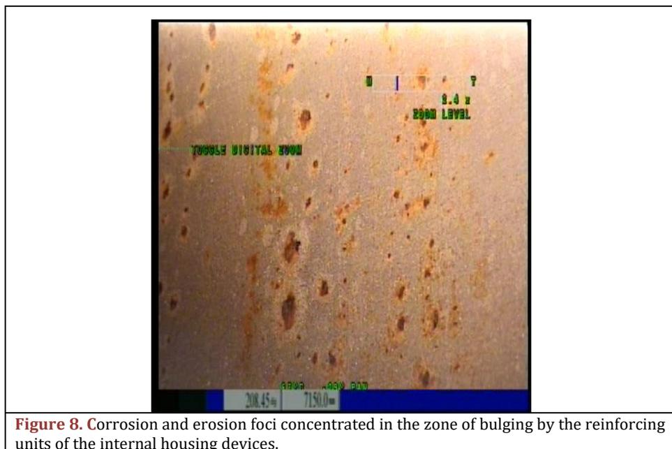
**Figure 8.** Corrosion and erosion foci concentrated in the zone of bulging by the reinforcing units of the internal housing devices.
