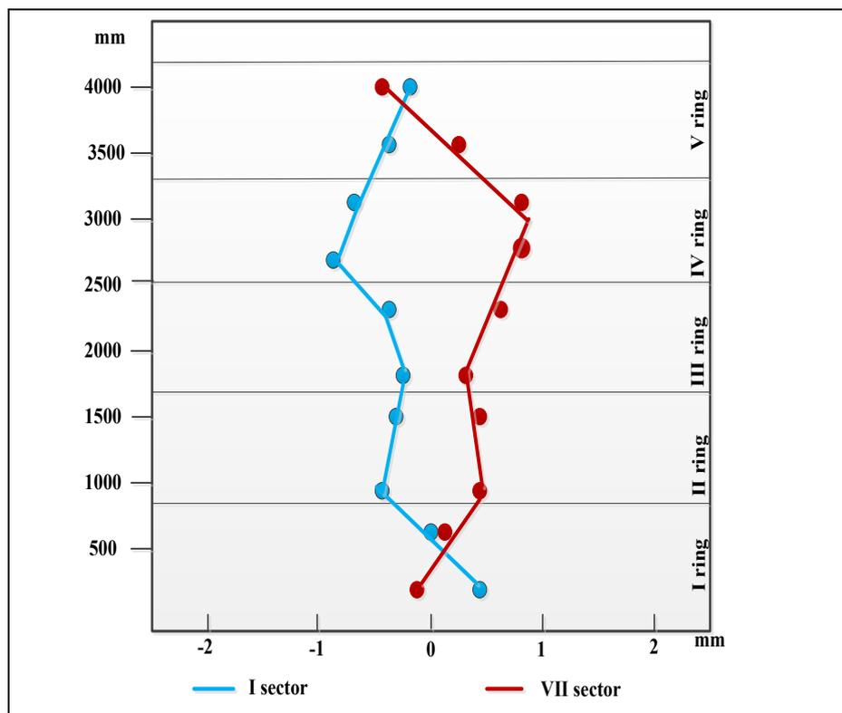
**Figure 11.** The sectors with maximum displacement are I and VII; the displacement dimensions are less than 1 mm.
