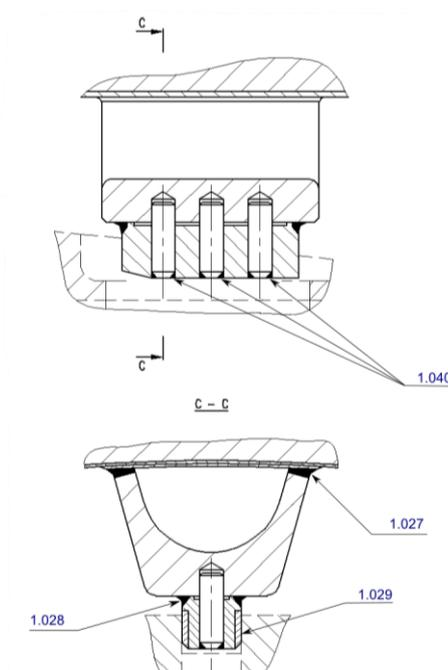
**Figure 4.** Core barrel fixation in RPV (key - groove and tongue).
