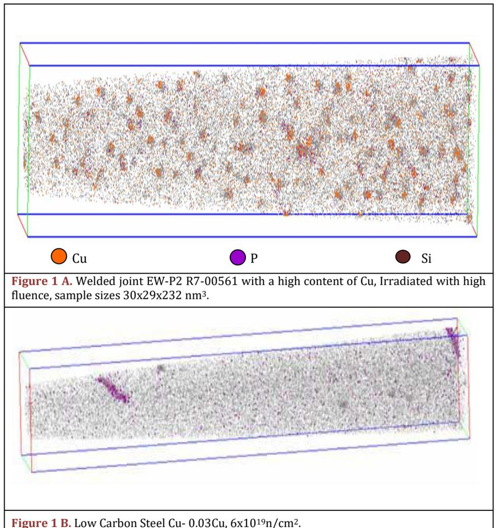
The uneven metal structure is the root cause of the brittleness of RPV Internals metals. (In the state of brittle fracture, metal fracture can occur suddenly and unpredictably, with a small influx of external energy). The neutron flux produced by the chain
