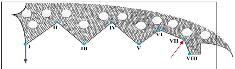
**Figure 10.** The areas with maximum displacement and the direction of displacement (with arrows).
