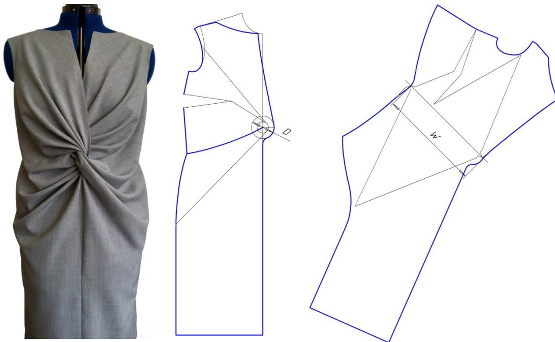
Figure 1. Design and pattern making of a lady's dress with a rich volume twist knot drapery [1].
