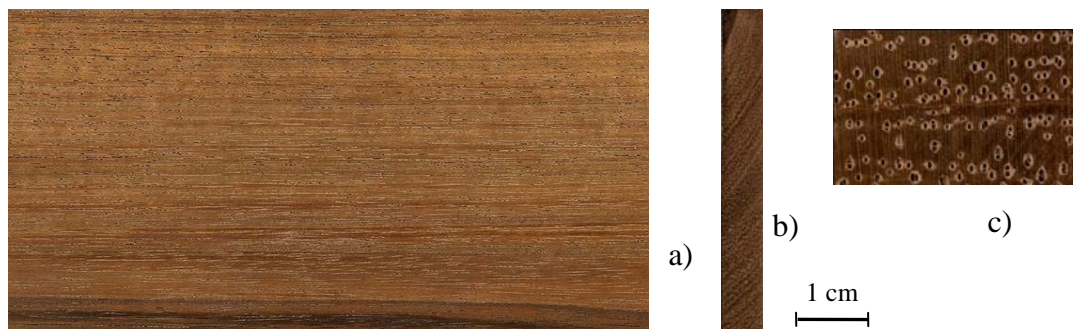
Fig.1. Flatsawn (a), quartersawn (b) surfaces of Tzalam wood sample, and an end grain view (c) of Tzalam (x 10).
