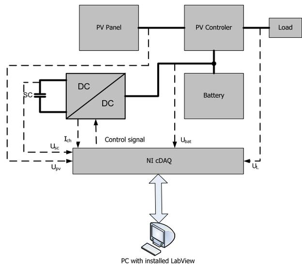
Fig.1. Block diagram of the stand for testing
