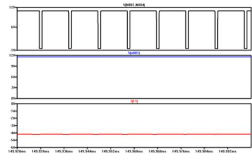
Fig. 6. Simulation results of the work of the converter in discharging mode
