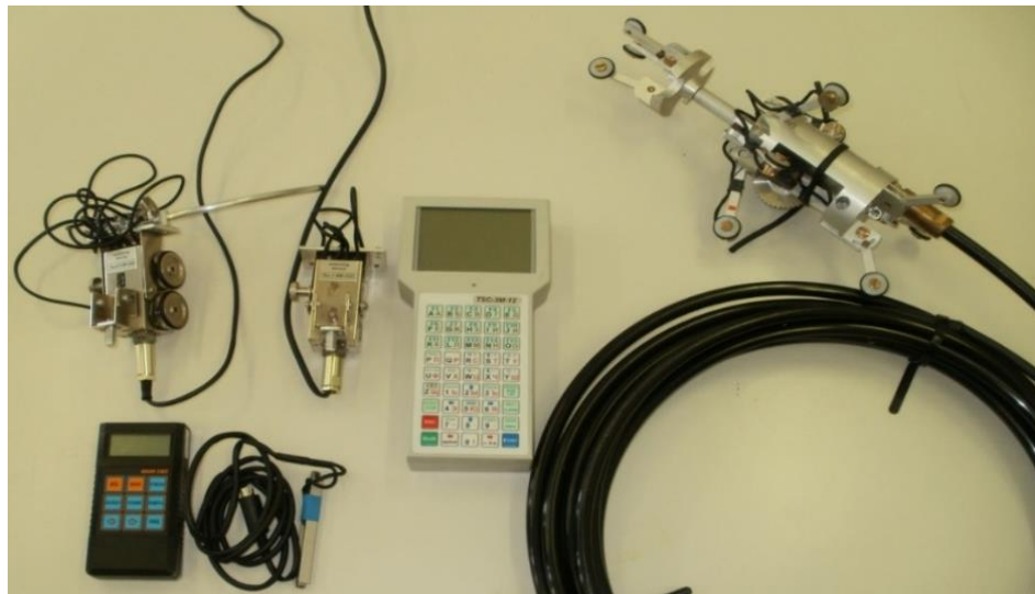
Fig. 2. Technical devices used by the metal magnetic memory method.
