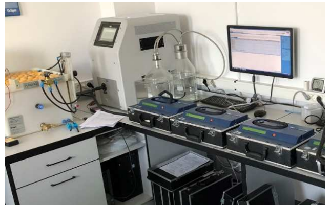
Fig. 1. Technical means used in examination and verification evidential breath analysers, type Alcotest 7110 Evident MK III
