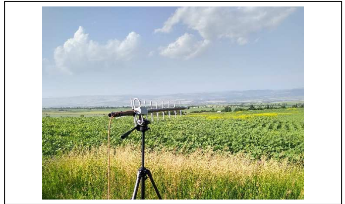
Fig. 10. The Yagi Antenna on a tripod, connected to the base station
