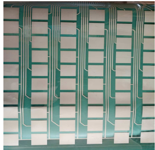
Fig. 2. Construction of the electrode sheet.
