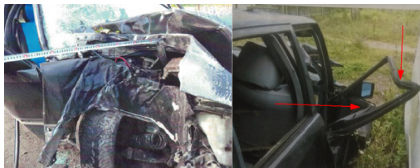
Figure 3. Deformations on the automobile.
