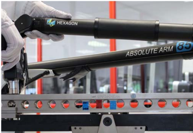
Fig. 5. Measurement with PCMM with certified standards
