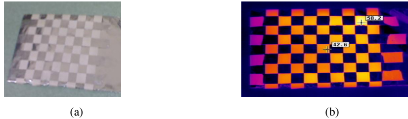
Fig. 3. (a) Test pattern Visual view. (b) Thermal image view
