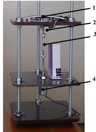
Fig. 3 Test bench 1 - digital display; 2 - weight sensors 3 –spring; 4 – solenoid type electromagnet.
