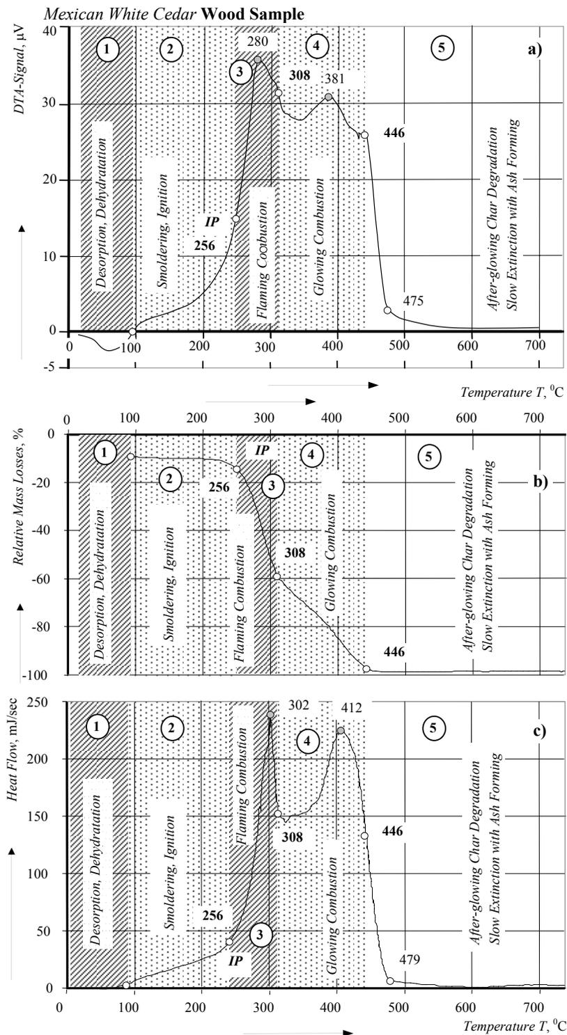
**Fig. 3.** Thermal analysis - DTA, TGA and DSC-spectra of bare *White Cedar* wood (*Cupressus Lusitanica*, Yucatan, Mexico) samples in air (heating rate:  $10\ ^\circ\text{C}$  per minute): wood pyrolysis stages identification (1, 2, 3, 4 and 5): **a** - by DTA-spectrum; **b** - by TGA-spectrum; **c** - by DSC-spectrum.
