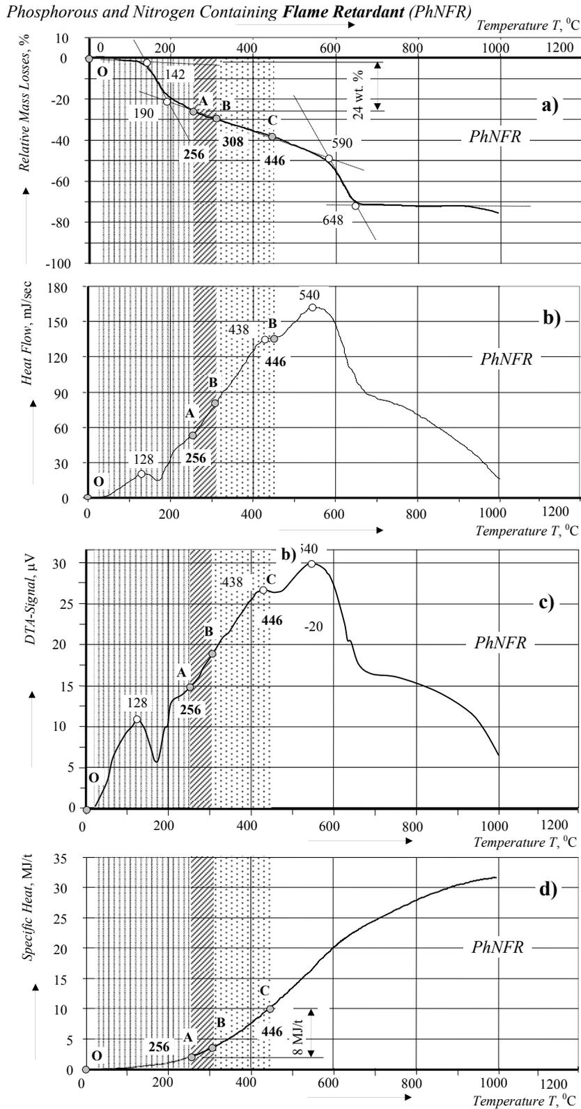
**Fig. 4.** Thermal analysis - TGA, DSC and DTA-spectra of bare phosphorous and nitrogen containing flame retardant (*PhNFR*) dried sample in air (heating rate: 10 °C per minute) in the temperature area of flaming and glowing wood pyrolysis stages (A-B-C): **a** - TGA-spectrum; **b** - DSC-
