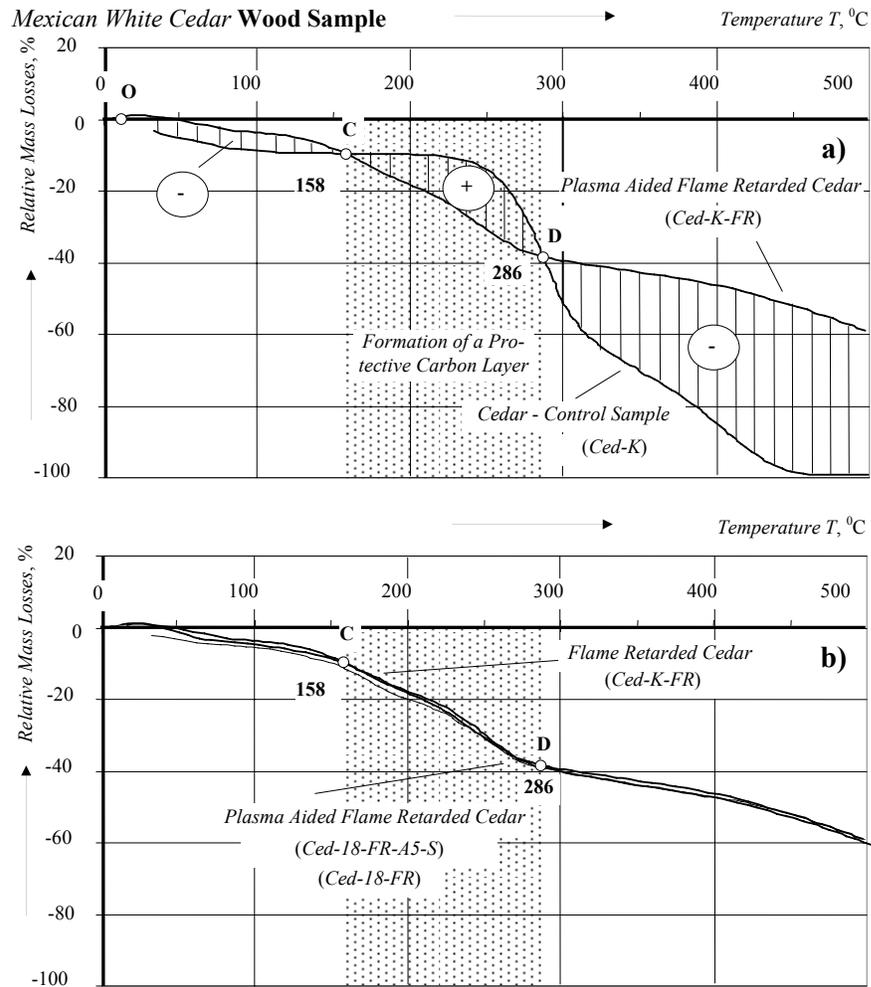
**Fig. 5.** Thermal TGA-analysis: flame retardency effect illustrated by the difference between relative mass losses demonstrated by bare (*Ced-K*) White cedar (*Cupressus Lusitanica*, Yucatan, Mexico) samples, flame retarded (*Ced-K-FR*) samples (**a**) and plasma-flame retarded wood (*Ced-18-FR*; *Ced-18-FR-A5-S*) samples (**b**) during air flow pyrolysis in the temperature interval up to 500 °C shown by DSC spectra (heating rate: 10 °C per minute).
