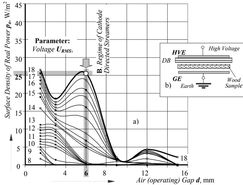
**Fig. 2.** Dielectric barrier air discharge (DBD) in asymmetric coplanar electrode system with one (alkali glass) barrier (a), technological discharge characteristic " $p_a - U_{RMS}$ ", and pick and choose regime (b) of plasma pre-treatment at industrial frequency and 18 kV (RMS).
