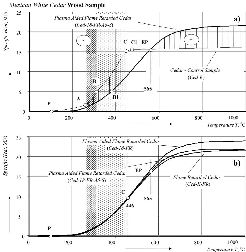
**Fig. 7.** Thermal analysis: *integral flame retardency effect* illustrated by the difference between released specific (per unit mass of sample) heat demonstrated by bare (*Ced-K*) *White cedar* (*Cupressus Lusitanica*, Yucatan, Mexico) samples, flame retarded (*Ced-K-FR*) samples (a) and plasma-flame retarded wood (*Ced-18-FR*; *Ced-18-FR-A5-S*) samples (b) during air flow pyrolysis in the temperature interval up to 1 000 °C takes by TGA and DSC spectra (heating rate: 10 °C per minute).
