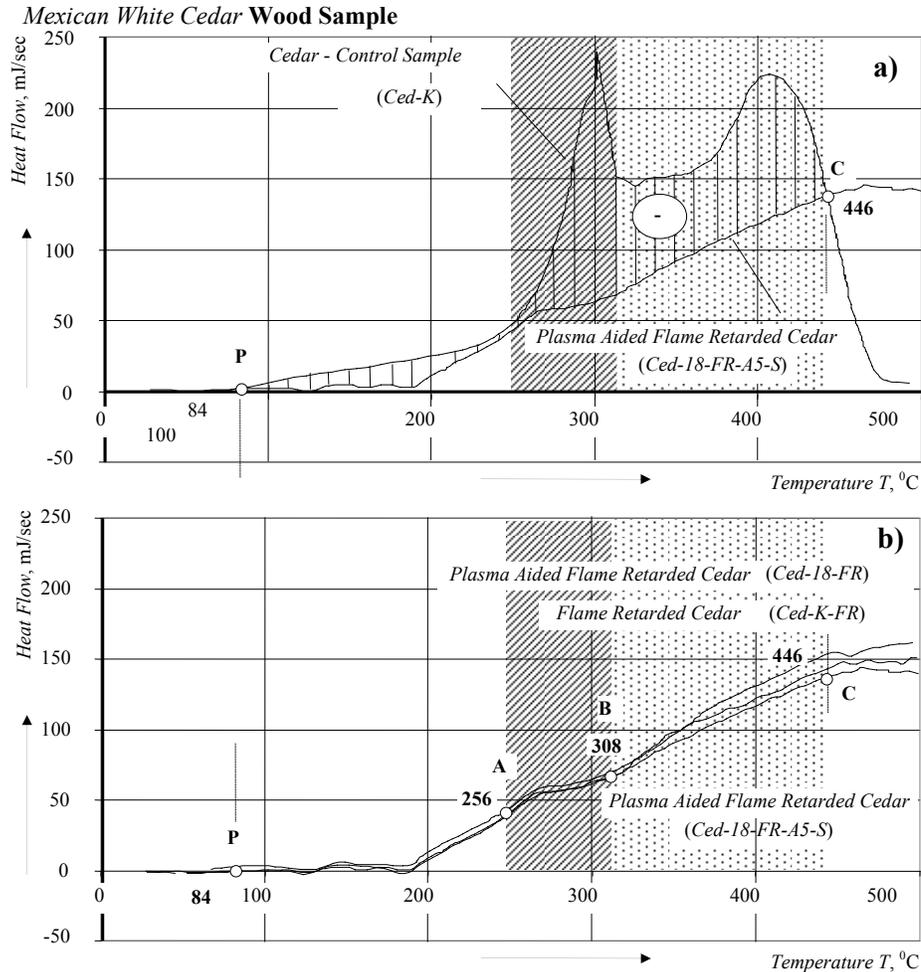
**Fig. 6.** Thermal DSC-analysis: flame retardency effect illustrated by the difference between heat flows demonstrated by bare (*Ced-K*) *White cedar* (*Cupressus Lusitanica*, Yucatan, Mexico) samples, flame retarded (*Ced-K-FR*) wood samples (a) and plasma-flame retarded wood (*Ced-18-FR*; *Ced-18-FR-A5-S*) samples (b) during air flow pyrolysis in the temperature interval up to 500 °C shown by DSC spectra (heating rate: 10 °C per minute).
