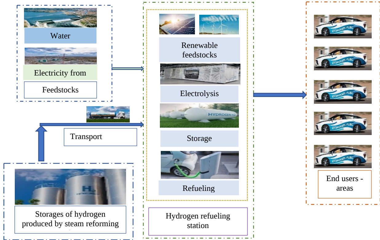
Fig. 2. A generalized superstructure of a hydrogen supply chain obtained through the electrolysis process
