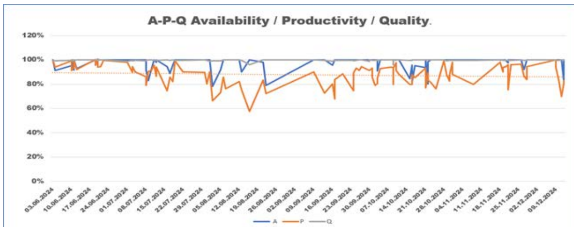
Fig.10 A-P-Q data for an automated assembly process.
