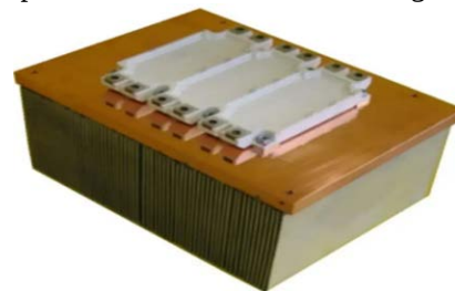
Fig. 4. Air-cooled radiator with copper base
