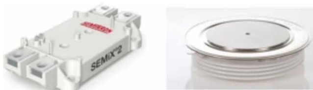
Fig. 2. IGBT packages for single-sided and double-sided cooling
