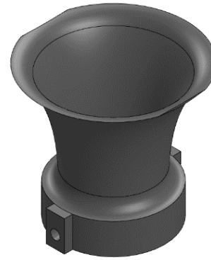
Fig. 3. Image of the modelled velocity stack within the environment of the software product SolidWorks.
