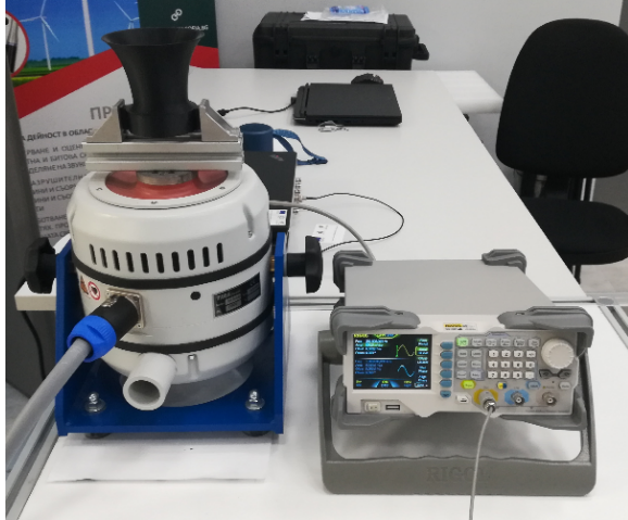
Fig. 8. Photo of the experimental setup with mounted velocity stack on the exciter.
