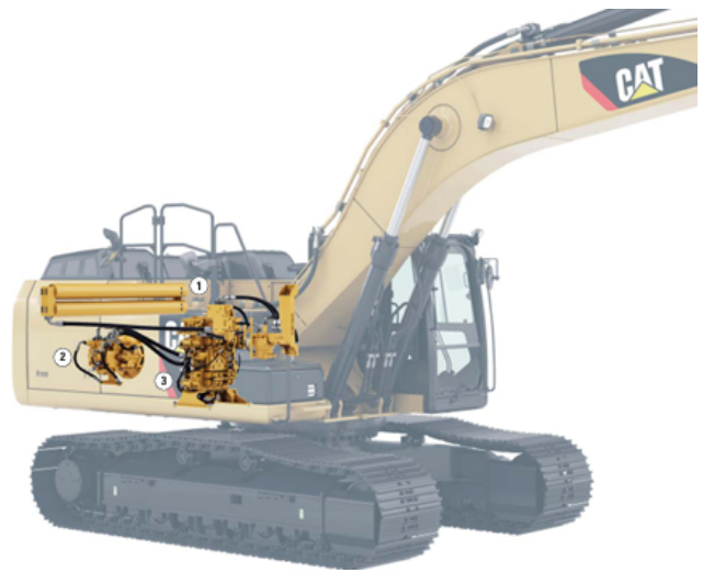
Fig. 3. Scheme of CAT 336 hybrid hydraulic system [8]. 1 – Hydraulic hybrid swing system; 2 – Electronic standardized programmable pump; 3 – Adaptive control system.
