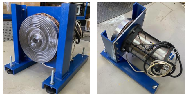
Fig. 10. Assembled physical prototype of developed AFIM.
