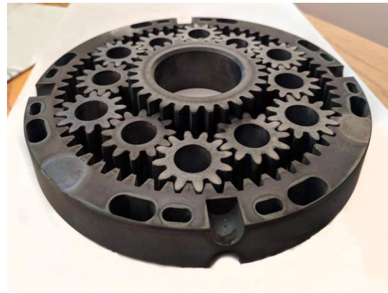
Fig. 14. Manufactured prototype gearing for a full planet engagement gear train
