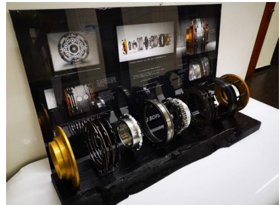
Fig. 15. Exploded showcase assembly of the full planet engagement differential developed for TU Sofia Racing team
