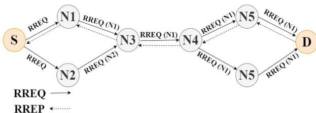
Fig. 9. Build up the reverse-path process
