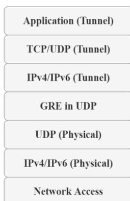
Fig. 1. The structure of GRE in UDP [9]
