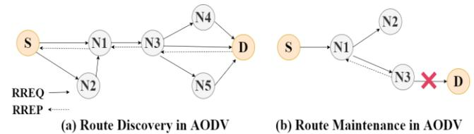
Fig. 8. Route discovery and Route maintenance in AODV
