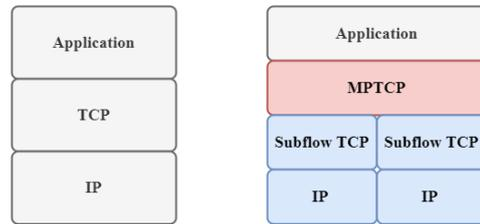
Fig. 6. Comparison between standard TCP and MPTCP [12]
