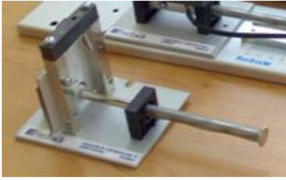
Fig. 7. Capacitive transducer with change of the distance between the plates
