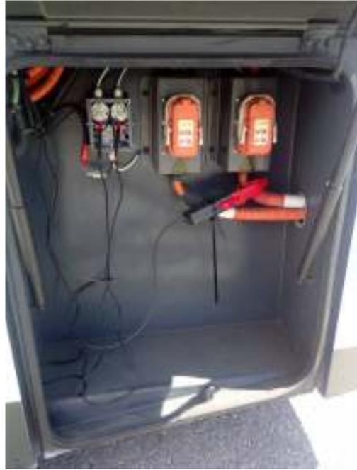
Fig. 4 connection to the RESS.
