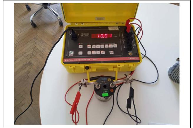
Fig. 2. Measuring the nominals of the reference resistors
