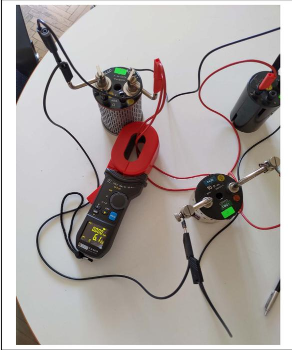
Fig. 4. Elongated hole Clamp-on measurement instrument CA 6118
