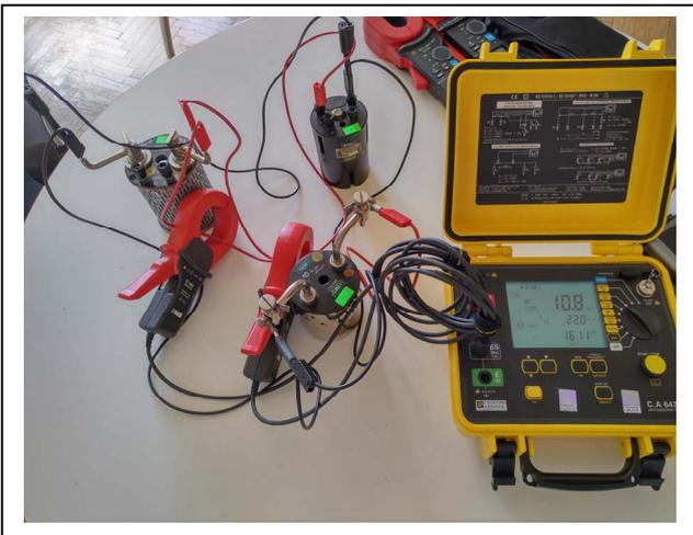
Fig. 5. Two clamps instrument CA 6472
