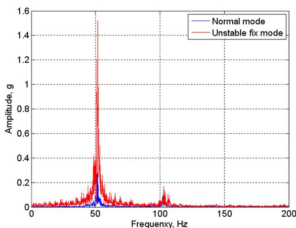
Fig. 10 Spectral analysis of the electrical motor vibrations.
