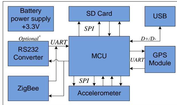
Fig. 5 Block diagram of the acceleration measurement end-device.
