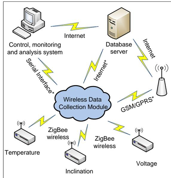
Fig. 1 Structure of the wireless measuring system.
