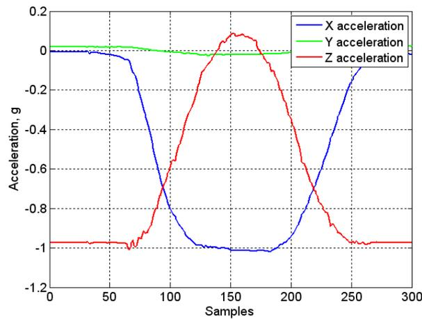
Fig. 9 Platform inclination (3-axis acceleration) measuring results.
