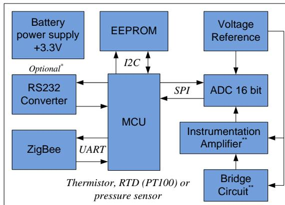
Fig. 3 Block diagram of a temperature measurement end-device.
