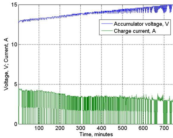
Fig. 8 Time diagrams illustrating the charge of a 12 V lead-acid accumulator battery.
