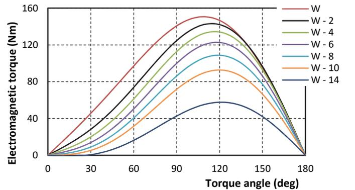
Fig. 3. Comparison of total electromagnetic torque characteristics at current 180A for different PM width and height  $H$ .
