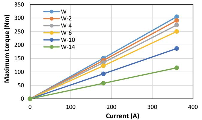
Fig. 6. Characteristics of the maximum torque depending on the current for different PM width and height  $H$ .
