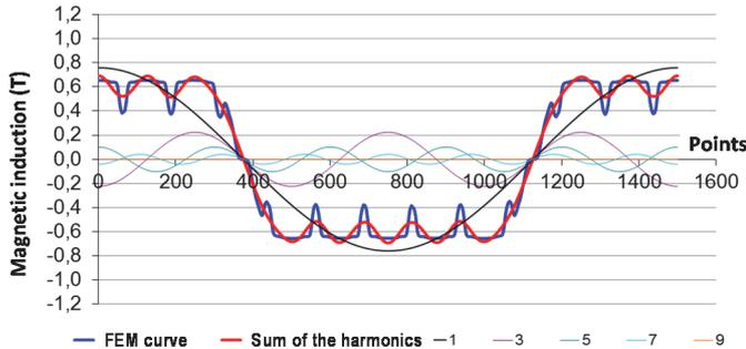
Fig. 12. Distribution of magnetic flux density created by PM with dimensions  $W \times H$ .
