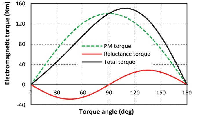
Fig. 2. Characteristics of electromagnetic torque and its components at current 180A for the base construction – PM width  $W$  and height  $H$ .
