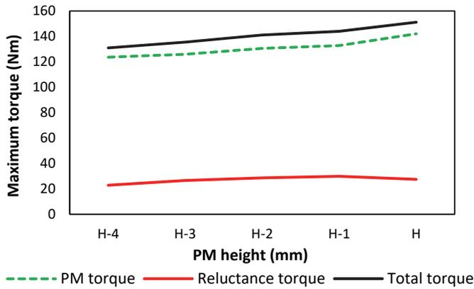
Fig. 9. Dependence of maximum values of torque components and total torque on PM height at current 180A and PM width  $W$ .
