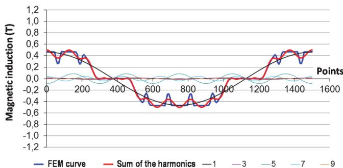
Fig. 13. Distribution of magnetic flux density created by PM with dimensions  $W-8 \times H$ .
