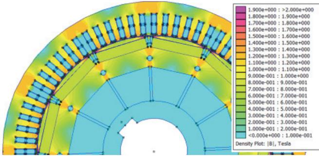
Fig. 1. Distribution of magnetic flux density in a PMSM with base construction – PM width  $W$  and height  $H$ .
