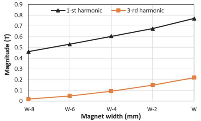
Fig. 14. Magnitude of the first and third harmonics of the magnetic induction created by the permanent magnets at a constant height  $H$  and different width.
