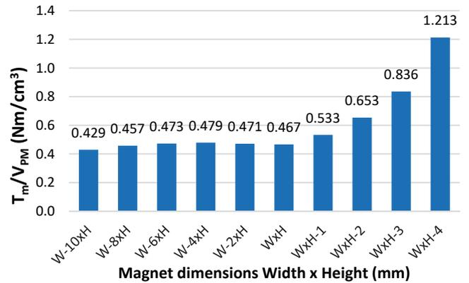
Fig. 11. Ratio of the maximum torque to the volume of the magnets at different dimensions of the PM and current of 180A.
