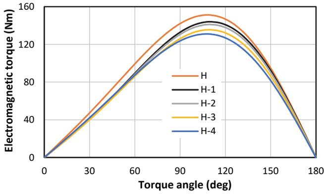
Fig. 8. Electromagnetic torque characteristics at current 180A, PM width  $W$  and different PM heights - from  $H$  to  $H-4$ .
