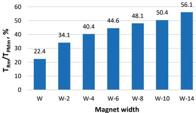
Fig. 5. The ratio of reluctance torque to PM torque at current 180A and PM height  $H$ .
