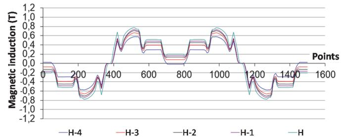
Fig. 15. Distribution of the air gap magnetic induction at PM flux weakening at different PM height and current of 180A.
