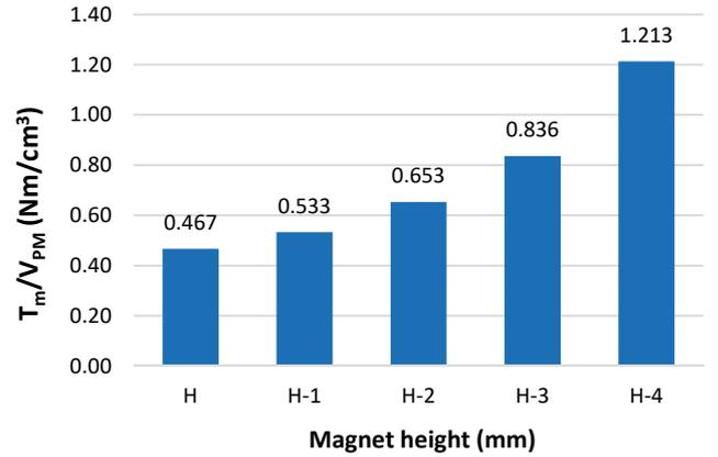
Fig. 10. Ratio of the maximum torque to the volume of the magnets when changing the PM height at constant width  $W$  and current of 180A.
