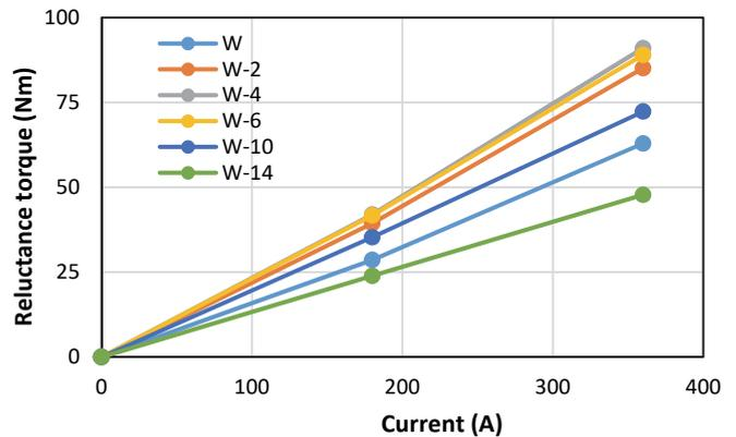
Fig. 7. Characteristics of the reluctance torque depending on the current for different PM width and height  $H$ .
