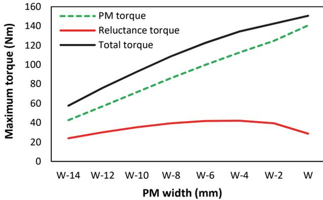
Fig. 4. Dependence of maximum values of torque components and total torque on PM width at current 180A and PM height  $H$ .
