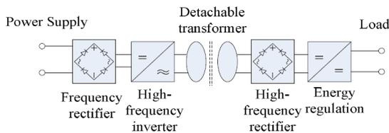
Fig. 2. The main blocks of the inductive charger [7]
