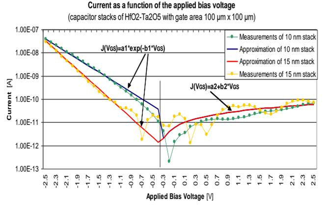
Figure 9.  $I$ - $V$  measurements vs. the proposed approximations for 10 nm and 15 nm capacitor stacks from  $\text{HfO}_2$ - $\text{Ta}_2\text{O}_5$  (y-axis is in logarithmic scale).
