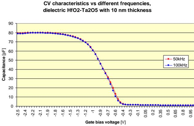
Figure 1.  $C$ - $V$  characteristics measured by RLC meter versus two frequencies across 10 nm  $\text{HfO}_2$ - $\text{Ta}_2\text{O}_5$  capacitor stack.
