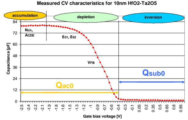
Figure 6.  $C$ – $V$  characteristics split into regions for fitting. In each region the corresponding parameters for fitting are shown.
