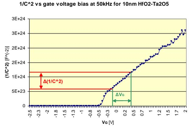
Figure 3. Curve of  $1/C^2$  vs.  $V_G$  at 50 kHz. It is observed the typical increasing slope after the onset of depletion.
