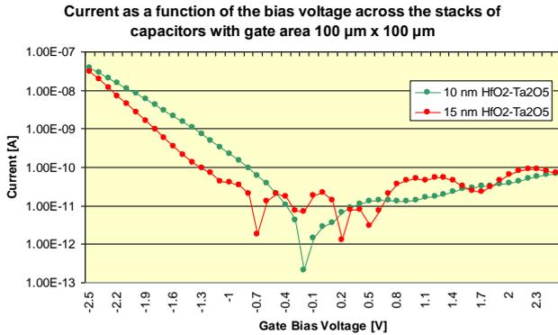
Figure 2.  $I$ - $V$  characteristics measured with Keithley 236 across 10 nm and 15 nm  $\text{HfO}_2$ - $\text{Ta}_2\text{O}_5$  capacitor stacks.
