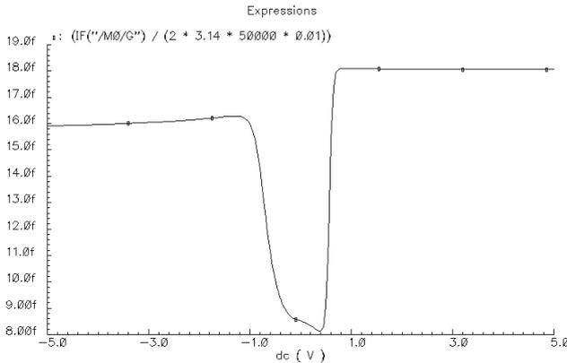
Figure 5.  $C$ - $V$  characteristics simulated by the capacitor-connected MOSFET model. The onset of strong inversion is observed after the threshold voltage.
