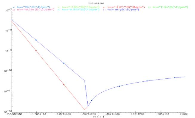
Figure 10.  $I$ - $V$  simulation vs. different dielectric thicknesses (the y-axis is in logarithmic scale). The curves is according to the characterization results.
