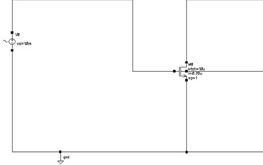
Figure 4. Bench circuit for simulation of  $C$ - $V$  characteristics of capacitor-connected MOSFET.
