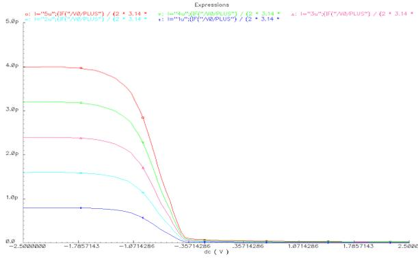
Figure 7.  $C$ - $V$  simulations vs. different values of the gate length. The characteristics performance matches theoretical expectations.
