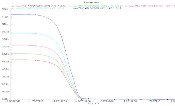
Figure 8.  $C$ - $V$  simulations vs. different values of the dielectric thickness. The characteristics performance matches theoretical expectations.
