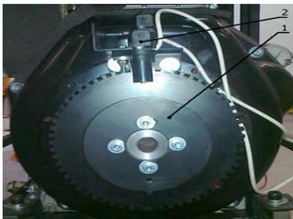
**Fig -2:** Location of the induction sensor for TDC
