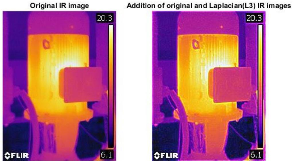
Figure 9. Original thermographic image and resultant image obtained by using Laplacian  $L_3$  high-pass filter.
