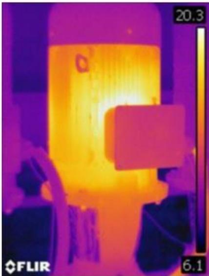
Figure 2. Thermographic image after application of the Gaussian low-pass filter.
