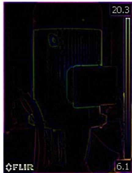
Figure 5. Thermographic image after application of the Laplacian  $L_1$  high-pass filter.
