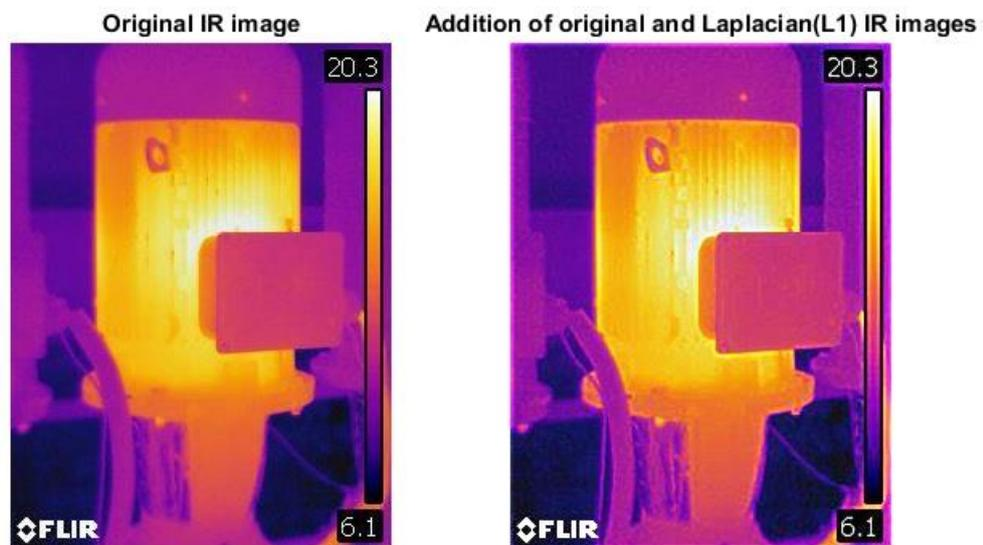
Figure 8. Original thermographic image and resultant image obtained by using Laplacian  $L_1$  high-pass filter.
