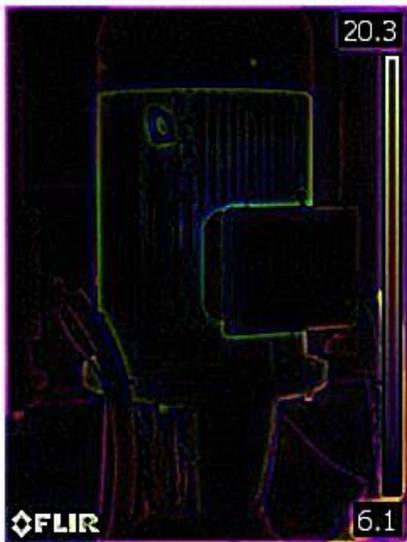
Figure 6. Thermographic image after application of the Laplacian  $L_3$  high-pass filter.
