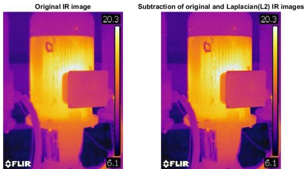
Figure 7. Original thermographic image and resultant image obtained by using Laplacian  $L_2$  high-pass filter.
