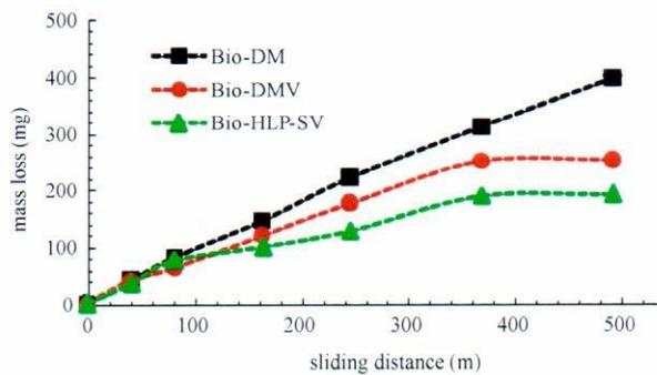
**Fig. 4.** Mass wear of the sample (counter-body) as a function of sliding distance
