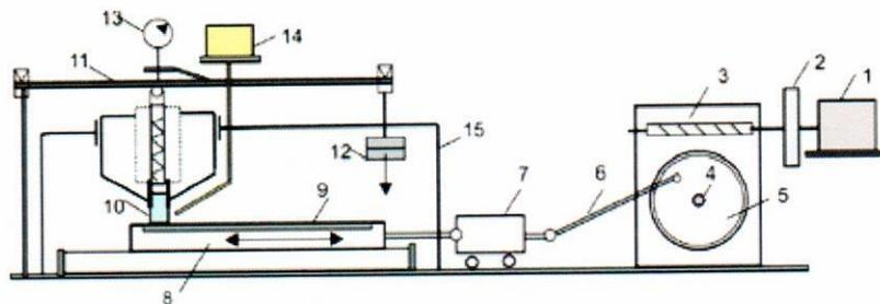
**Fig. 1.** Scheme of tribotester RT16 for studying the wearing off process in case of reverse-translation movement
