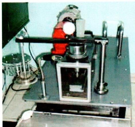
**Fig. 2.** Photograph of tribotester RT16 for studying the wearing off process in case of reverse-translation movement
