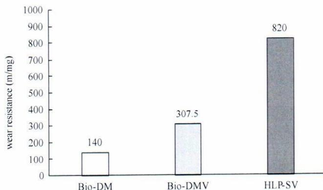
**Fig. 5.** Diagram of wear resistance of sample 10 (the body) made of instrumental steel during lubrication and sliding distance  $L = 492$  m
