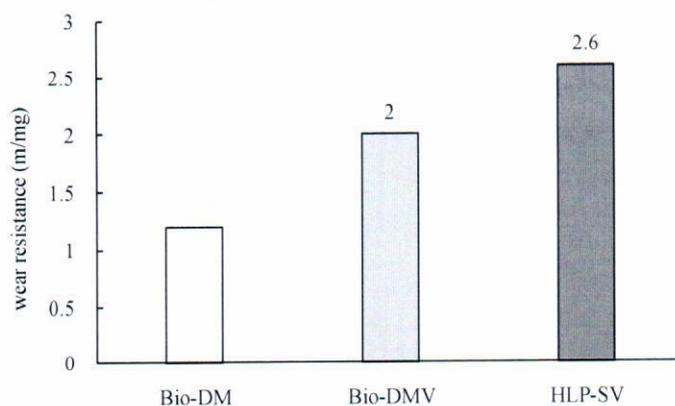
**Fig. 6.** Diagram of wear resistance of sample 9 (the counter-body) made of steel St3sp during lubrication and sliding distance  $L = 492$  m
