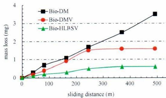
**Fig. 3.** Mass wear of the sample (body) as a function of sliding distance
