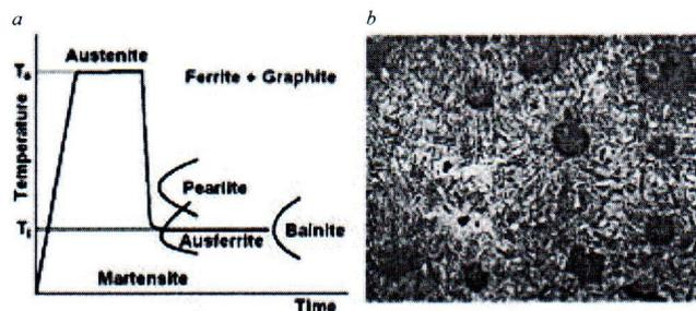
**Fig. 2.** Diagram of the isothermal procedure (a) and with bainite microstructure of nodular cast iron (b)
