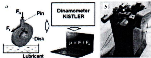
**Fig. 3.** Schematic view of research procedure (a) and image of the Tribometer 'Pin-on-Disk' TPD-93 (b)
