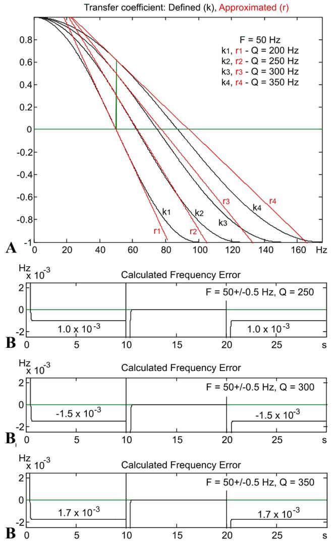
Fig. 2. Experiment with a “two-point” digital filter at  $q = 1$ .
