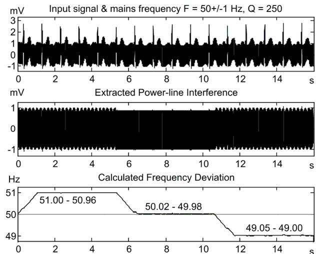
Test No 1: Signal ECGprobe,  $Q = 250$  Hz,  $F = 50 \pm 1$  Hz.
