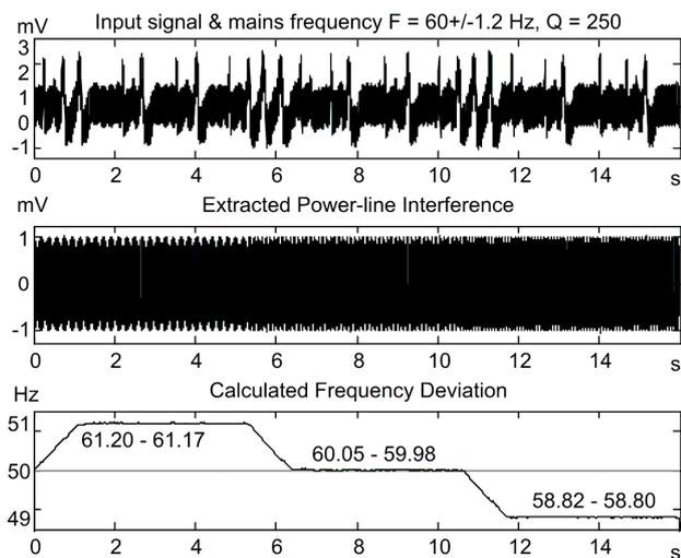
Test No 2: Signal AHA\_7009,  $Q = 250$  Hz,  $F = 60 \pm 1,2$  Hz.
