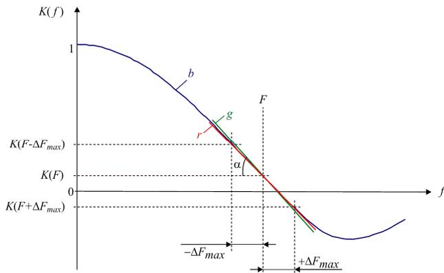
Fig. 1. Linear approximation of the digital filter frequency response in the range of mains frequency deviation.
