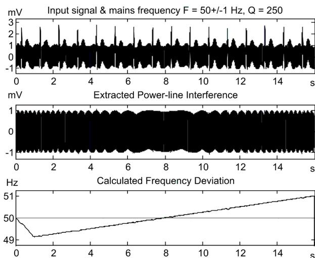
Test No 3: Signal ECGprobe,  $Q = 250$  Hz,  $F = 50 \pm 1$  Hz.
