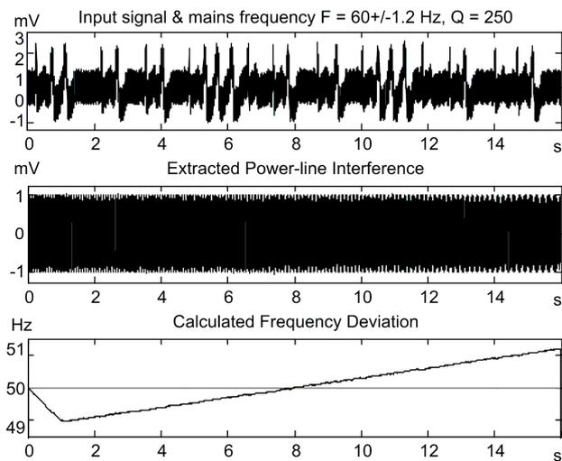
Test No 4: Signal AHA\_7009,  $Q = 250$  Hz,  $F = 60 \pm 1,2$  Hz.
