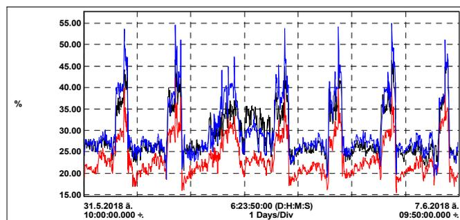
Fig. 11. Total harmonic distortion of the phase currents L1 – black; L2 – red; L3 – blue
