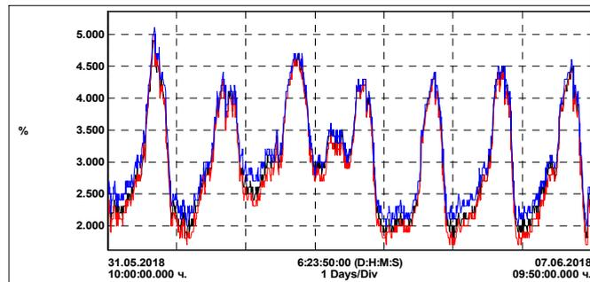
Fig. 9. Total harmonic distortion of the phase voltages L1 – black; L2 – red; L3 – blue
