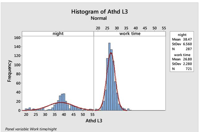
Fig. 12. Histograms of the total harmonic distortion of the phase currents
