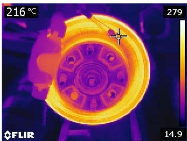
Fig. 6. FLIR thermal image of the rotating disk
