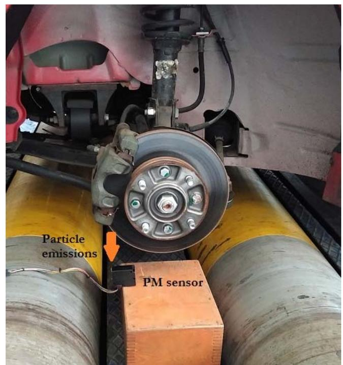
Fig. 1. Particulate measurement method and assembly
