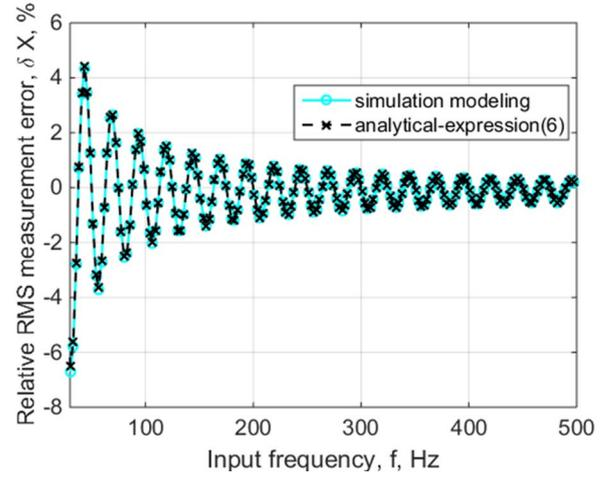
Fig. 1. The dependence of the RMS measurement error (moving averaging method) on the input signal frequency
