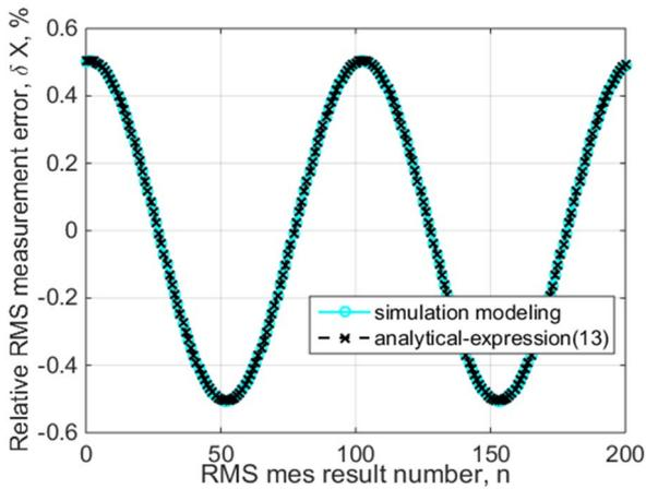
Fig. 2. The dependence of the RMS measurement error for the method of moving averaging on the number of measurement result
