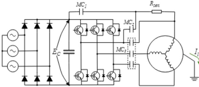
Fig. 1. Scheme for measurement of the insulation resistance via variable frequency drive
