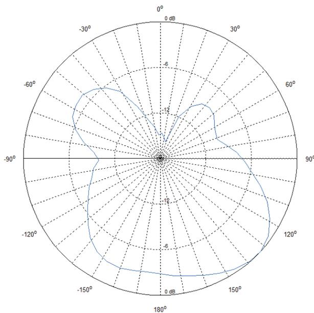
Figure 7. Experimental Radiation Pattern of AUT @ 433,92 MHz
