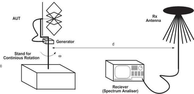
Figure 4 - Scheme of Test Stand for Radiation Pattern Measurements of 2biQUAD antenna in vertical plane
