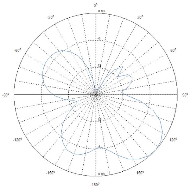
Figure 8 - Experimental Radiation Pattern of AUT @ 2,45 GHz
