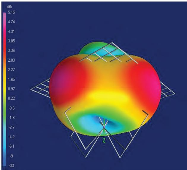
Figure 2 - 2biQUAD antenna simulated 3D radiation pattern
