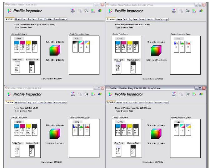
Fig.5 - Comparison of the basic parameters of the studied color profiles (factory-bottom left; i1Profiler - bottom right; Fiery Color Profiler - top right) versus standard offset profile Fogra 39 (top left)
