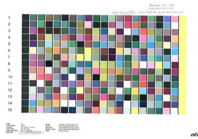
Fig.3 – Results from measurement and averaging of color values during profiling (mean Delta E2000 error = 0.6)
