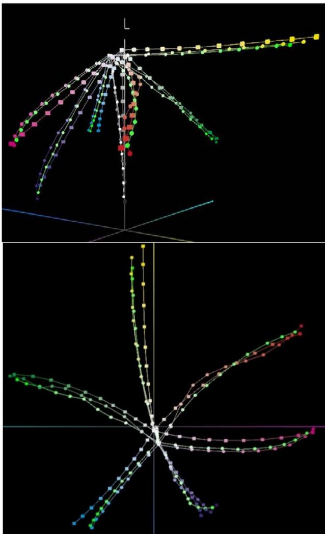
Fig.11 and 12 - Primary and secondary colors of i1Profiler generated profile (spheres); Fiery Color Profiler profile (green spheres) and offset profile Fogra 39 (cubes)
