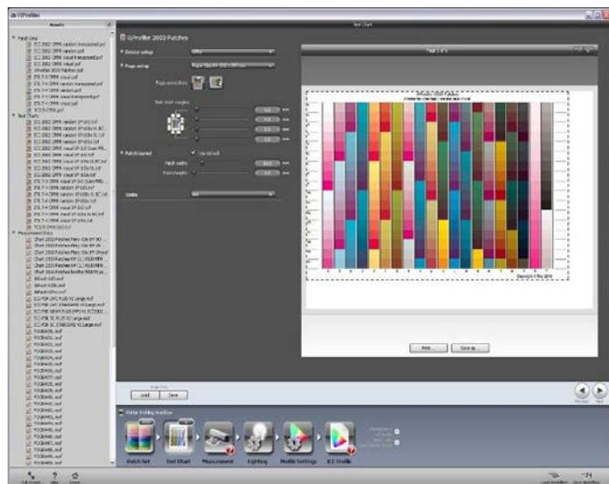
Fig.1 – Reference profiling target without color management as it will actually be printed and measured (only page 1 of 6 shown)
