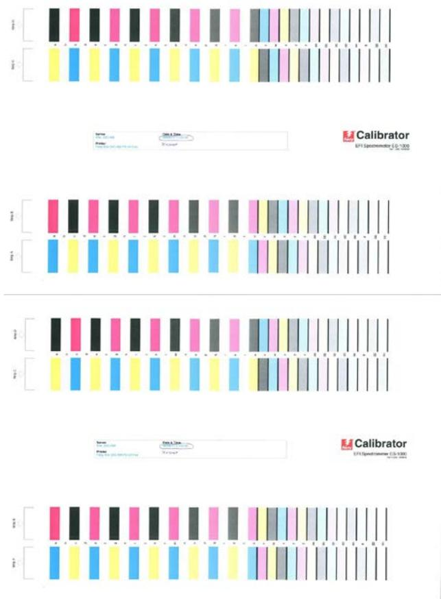
Fig.5 and 6 - Test page for calibration and linearisation of a C350 printer by a spectrophotometer with successive colors (top) and randomly arranged colors (bottom)
