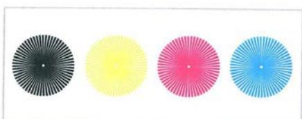
Figure 3 – Circular resolution test element printed on the Konica Minolta Bizhub C350
