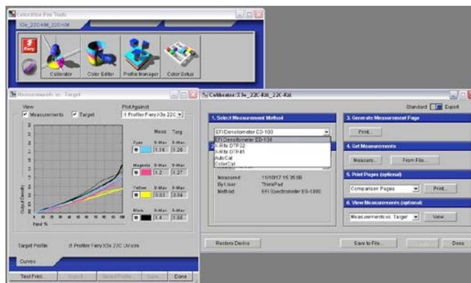
Fig.4 - Calibration menu for printer C350 (measured and set optical density at calibration)
